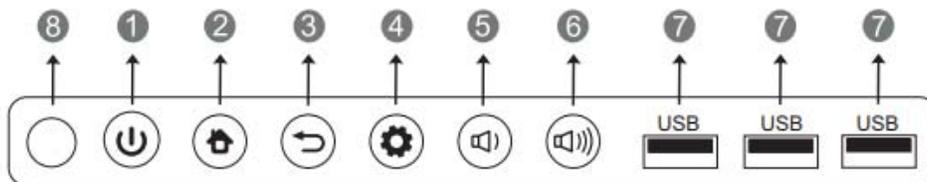
1. **Power** key, press to turn on – press and hold to turn off. Press to turn on/off the display backlight only.
